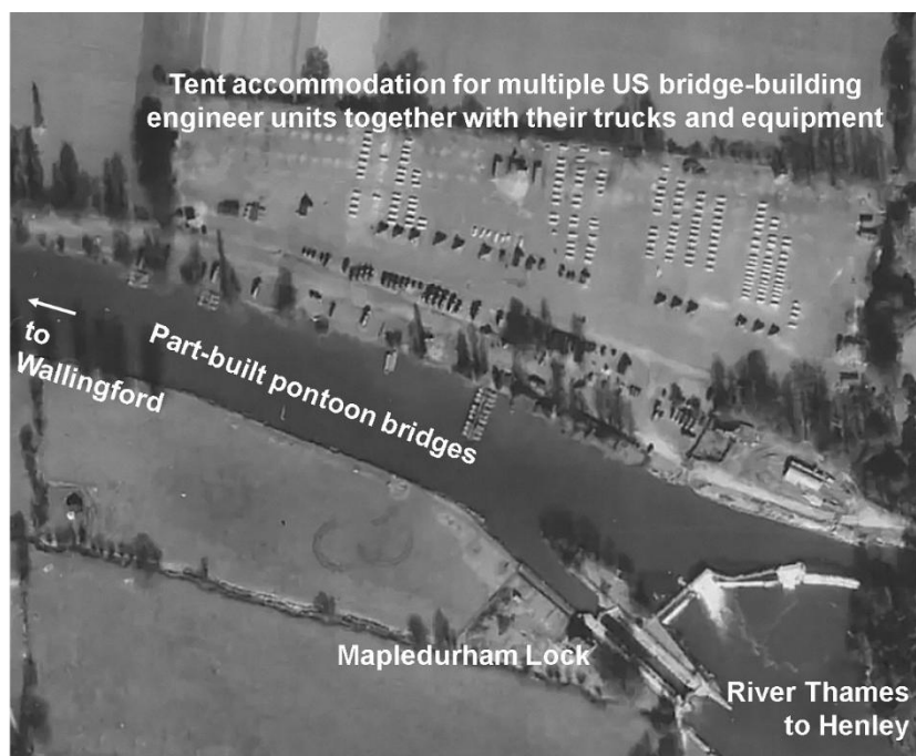
Figure 8: The river Thames at Mapledurham was extensively used by the US for bridge-building practice. This vertical aerial photograph was taken by the USAAF on 8 March 1944 and shows several part-built pontoon bridges. (Credit: Historic England, Aerial Photo Exp)
